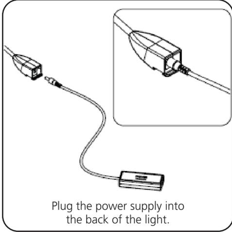
Plug the power supply into the back of the light.
