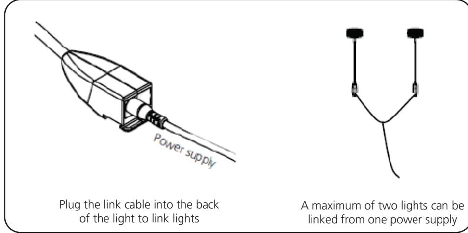
Plug the link cable into the back of the light to link lights
