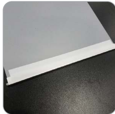
Take the re-enforcing tape and apply to the back of the banner and rail making sure there is even coverage between the two.
