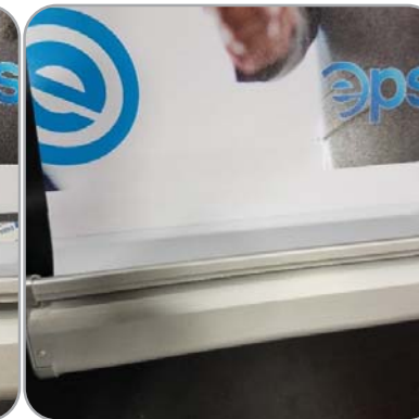
Mount graphic to leader strip evenly making sure there is one 1/2" of overlap.
